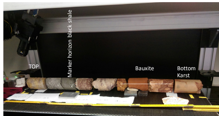
Figure 1. LIBS measurement configuration of composite bauxite profile.
