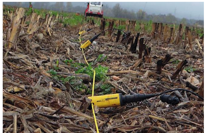
Field deployment for High-Resolution Vibro-Seis Survey
