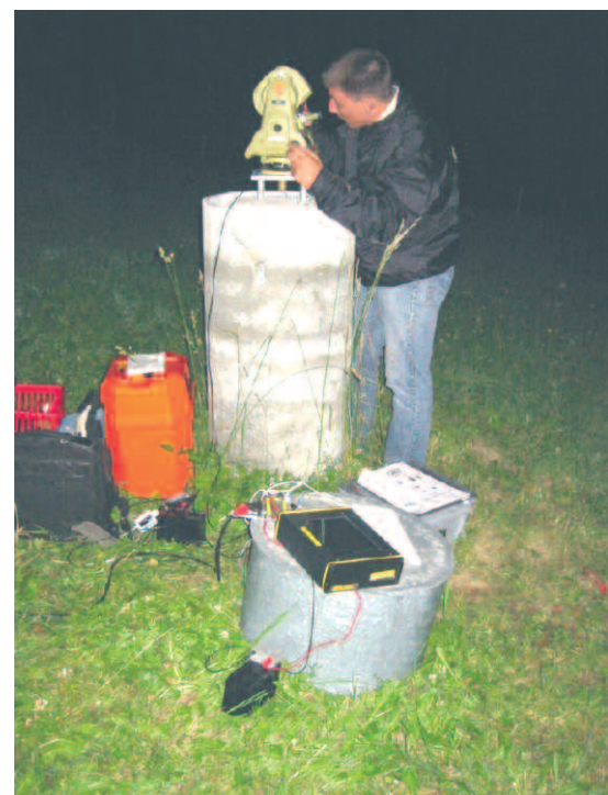
Fig. 4: Geomatic engineering student and co-author of the present article S. Guillaume, measuring an astro-geodetic azimuth between terrestrial mire and the polar star (alpha Ursae Minoris).
