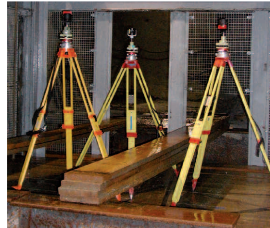
Fig. 5: Positioning of tripods at bottom of shaft.
