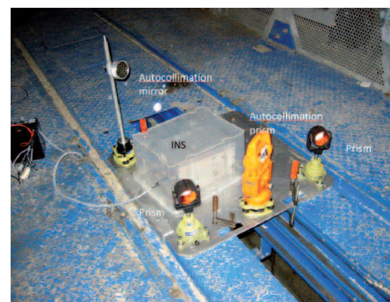
Fig. 5: Direction transfer using IMAR inertial navigation system.
