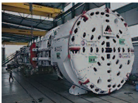
Fig. 4: Tunnel boring machine at the Herrenknecht plant
