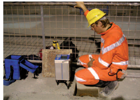
Fig. 4: Gravity measurements in the tunnel.
