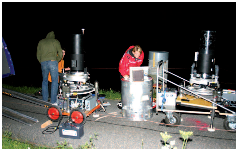
Fig. 5: The two zenith camera systems of the Leibnitz University of Hannover (left) and the ETHZ (right) during the survey at the Erstfeld portal pillar.
