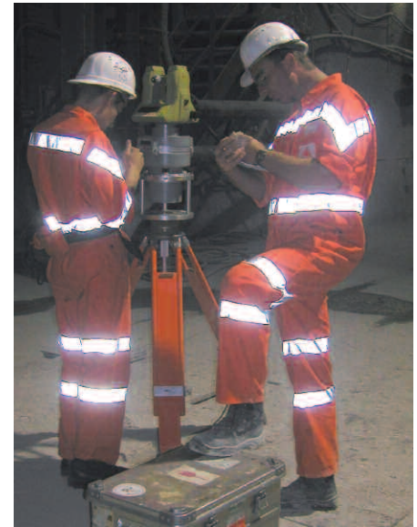
Fig. 5: Gyro measurements with GYROMAT 2000 , Instr. No. 225, version Unibw (wireless controlling, data transfer and evaluation with PDA).
