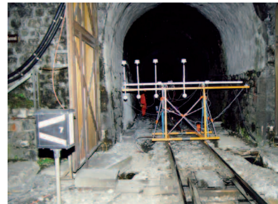
Fig. 3: Temperature gradient measurement system.
