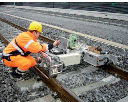
Fig. 3: Track gauging trolley RACER.
