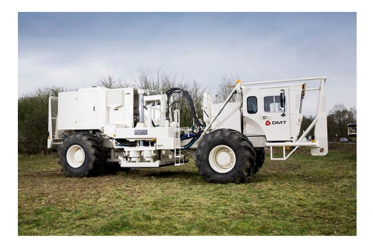
The Hemi 48 vibrator mounted on the M12 off-road chassis is an ideal seismic source unit if high quality results are needed from geophysical exploration.
